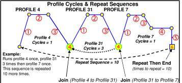
profile can be made to run itself 1 to 9999 times or continuously using the Profile cles setting. A profile ending with Repeat Then End will run the entire sequence profiles again 1 to 9999 times or continuously
