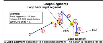
required number of times (1 to 9999) before the profile continues onwards. More an one Loop Segment can be used, but they must not cross.
