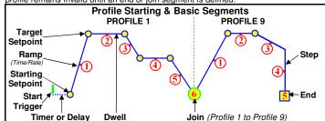
ollowing a Start Trigger, profiles can start immediately, after a delay, or from the imer (*Recorder only*)
